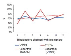
Figure 1: VTS and COD removal from swine manure-fed biodigesters. Source: Report from INRH, Cienfuegos.
