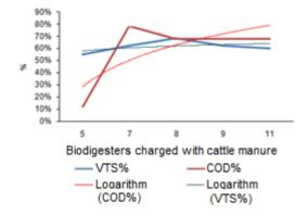
Figure 2: VTS and COD removal from cattle manure-fed biodigesters. Source: Report from INRH, Cienfuegos.
